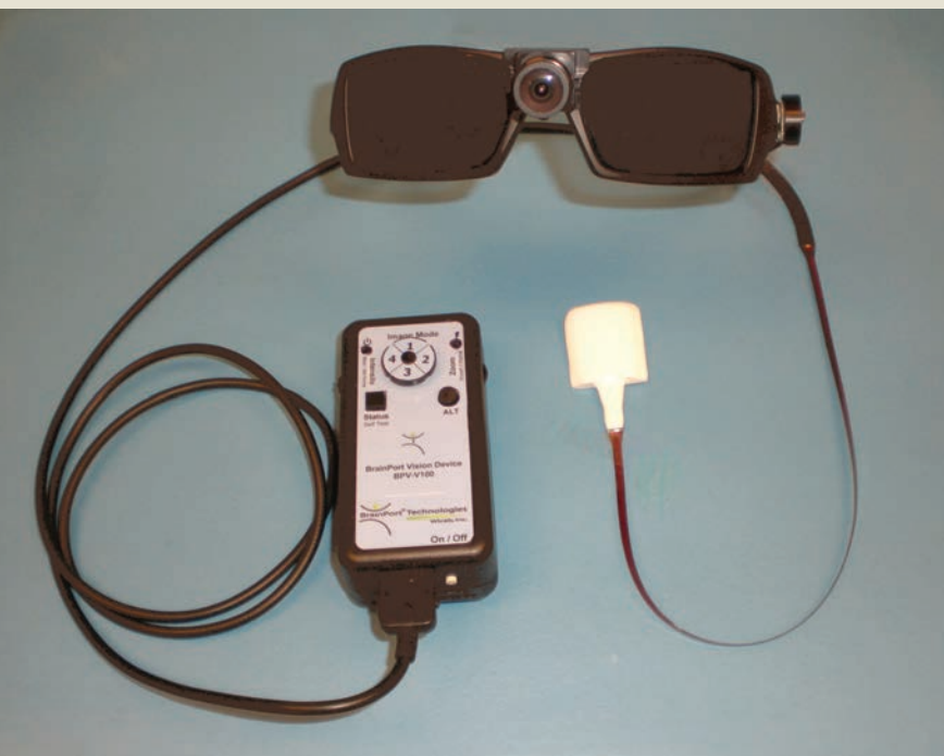
The lollipop-device uses the tongue to stimulate the visual cortex.
